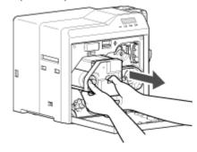
3 Cut away the broken portion, and attach the unused portion at the supply side to the other end at the take-up side using an adhesive tape, while making sure that the joint surface is even
