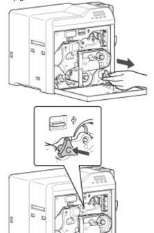
Turn the card feed roller shaft in the anti-clockwise direction, while checking the position of the card
