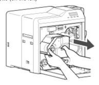
4 Apply alcohol to a cotton swab (large), and use it to wipe the four bobbin holders
