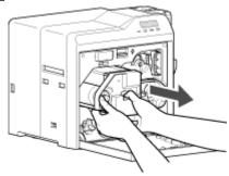
3 Attach the jog dial to the card feed roller shaft
