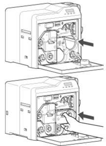
6 Press Reset → to reset the printer
