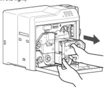
${\it 3}$  Press and hold down the cassette button, and remove the retransfer film cassette (on the left)
