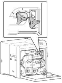
• If the card protrudes from the card turn over unit, turn the cleaning roller shaft to move the card into the unit.
