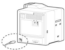
2 Plug the power cord (supplied) into an outlet
