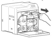
5 Remove the jammed card in the card turn over unit from the card load slot
