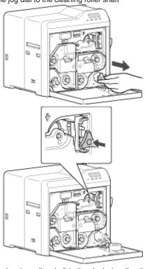
4 Turn the cleaning roller shaft in the clockwise direction, while checking the position of the card
