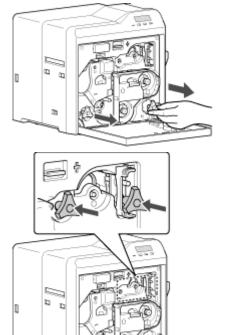
(4) Turn the card feed roller shaft and cleaning roller shaft in the clockwise direction, while checking the position of the card
