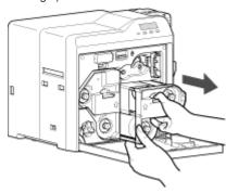
3 Press and hold down the cassette button, and remove the retransfer film cassette (on the left) to remove the retransfer film
