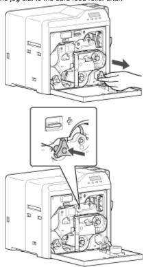
4 Turn the card feed roller shaft in the anti-clockwise direction, while checking the position of the card
