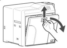
2 Press and hold down the cassette button, and remove the retransfer film cassette (on the left)
