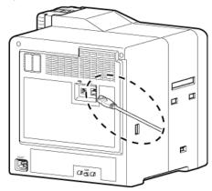
${\it 3}$  Plug the LAN cable into the connection terminal of the hub that is installed on the network that the computer is connected to
