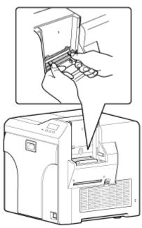
4 Open the printer door, and remove the cleaning unit
