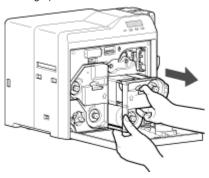
3 Cut away the broken portion, and attach the unused portion at the supply side to the other end at the take-up side using an adhesive tape, while making sure that the joint surface is even
