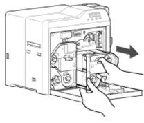
3 Press and hold down the cassette button, and remove the retransfer film cassette (on the left)
