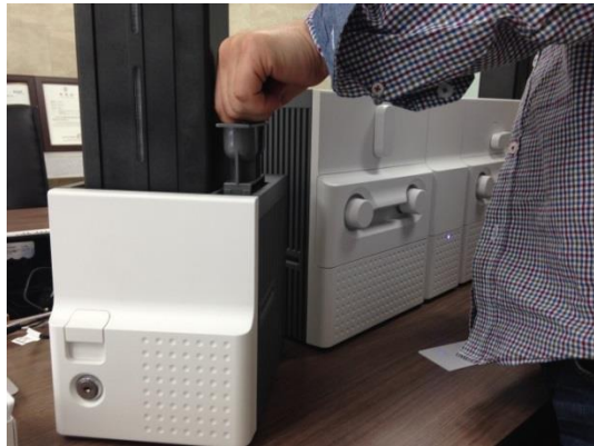
Figure 137 Input Hopper cleaning 2
