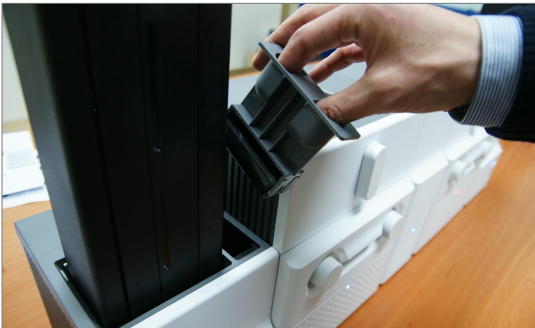
Figure 31 Installation of disposable cleaning roller holder
