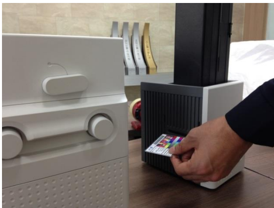
Figure 132 Card jam in Output Hopper 2
