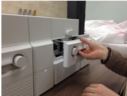
Figure 158 Laminator Head replacement 2
