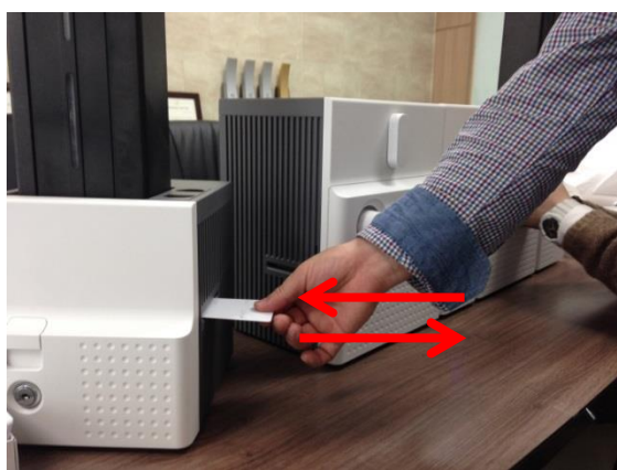
Figure 114 Card jam in Input Hopper 3
