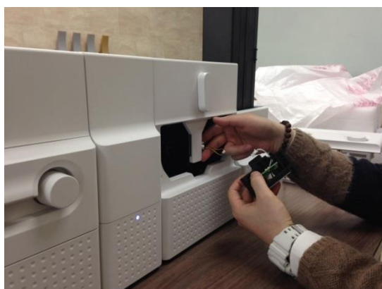
Figure 161 Laminator Head replacement 5
