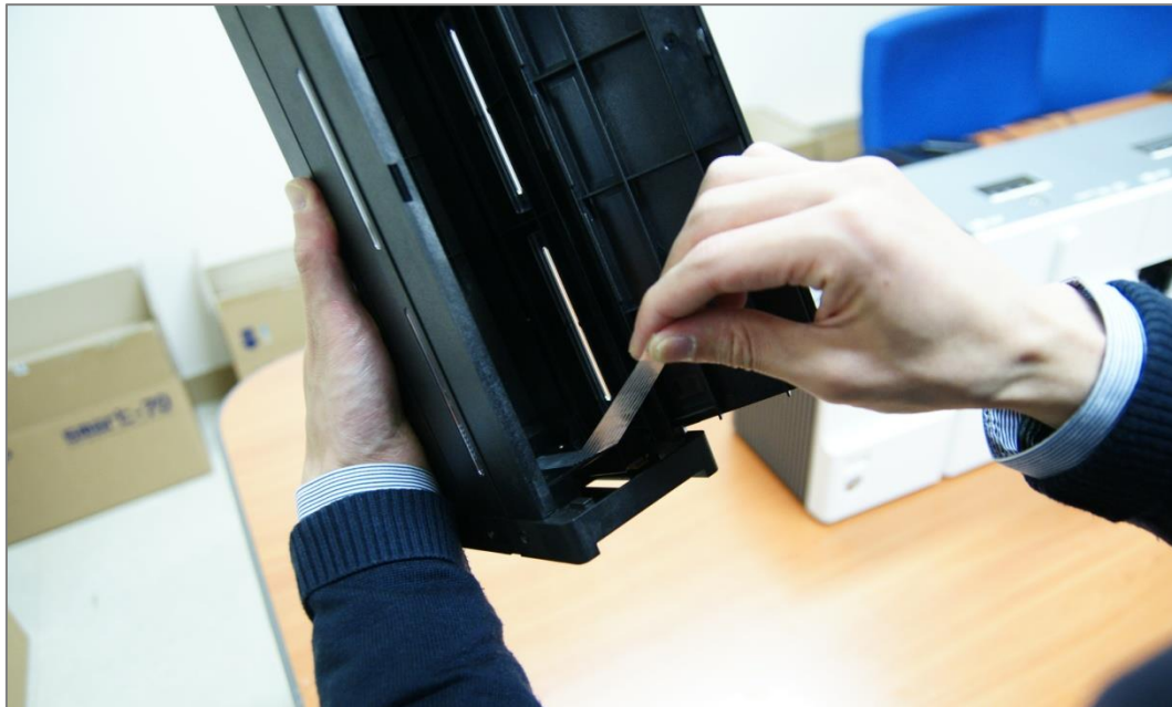
Figure 35 Removal of the tape for fixing the weight
