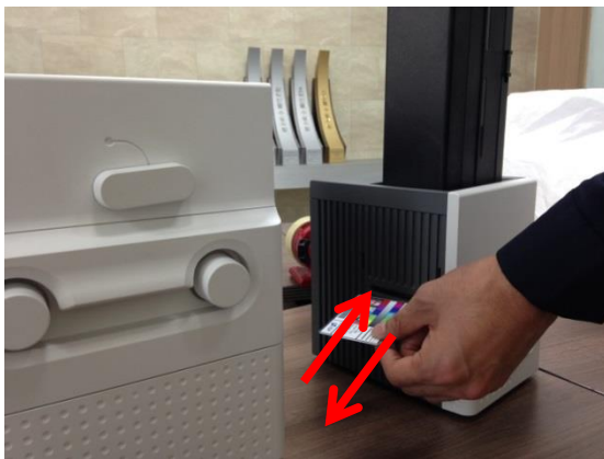
Figure 133 Card jam in Output Hopper 3
