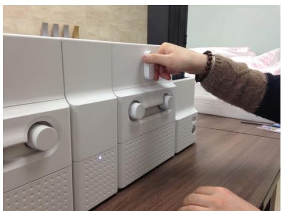
Figure 157 Laminator Head replacement 1
