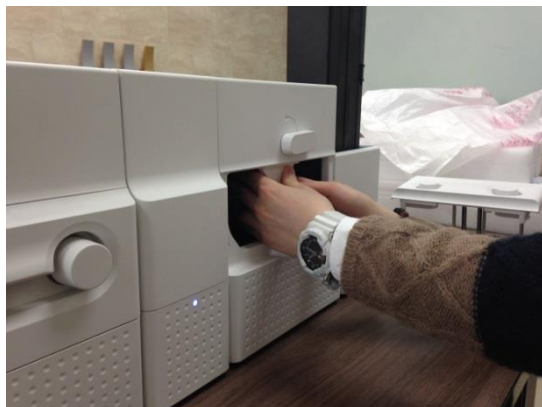
Figure 159 Laminator Head replacement 3
