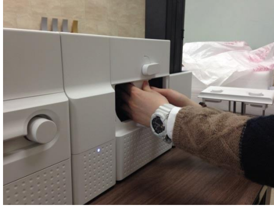
Figure 162 Laminator Head replacement 6
