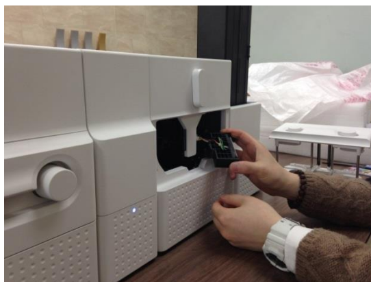
Figure 160 Laminator Head replacement 4
