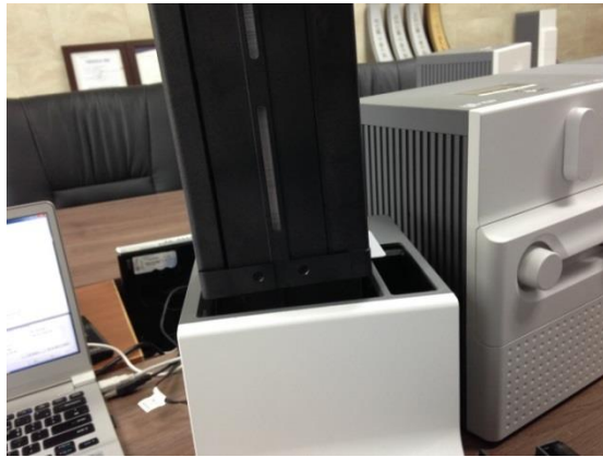
Figure 116 Card jam in Input Hopper 5
