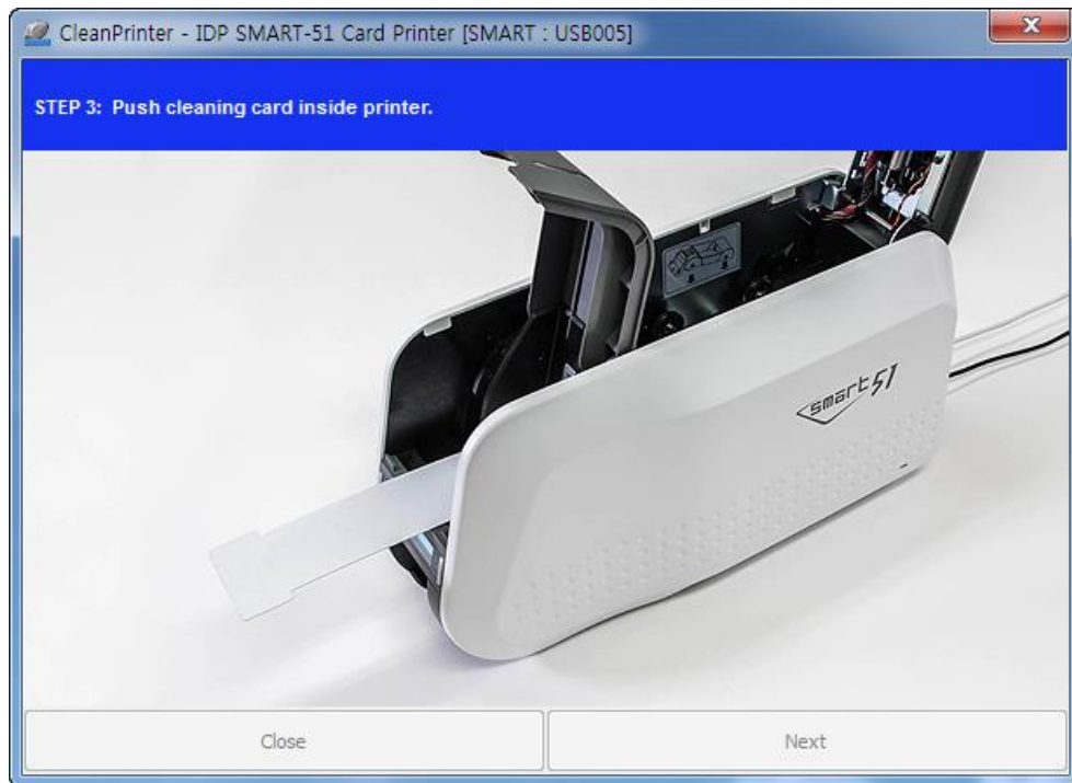
Figure 108 Printer cleaning Step 3
