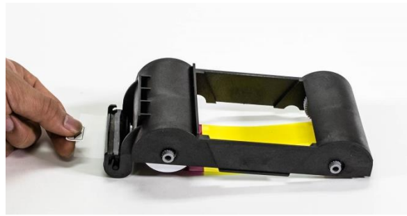
Figure 18 Peeling the protective wrapper
