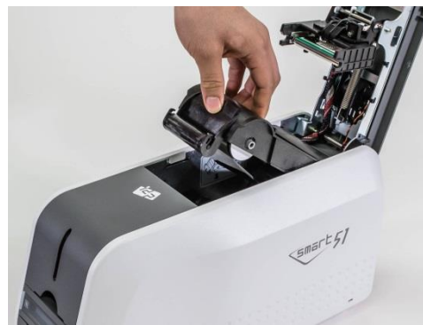
Figure 19 Installing the ribbon cartridge
