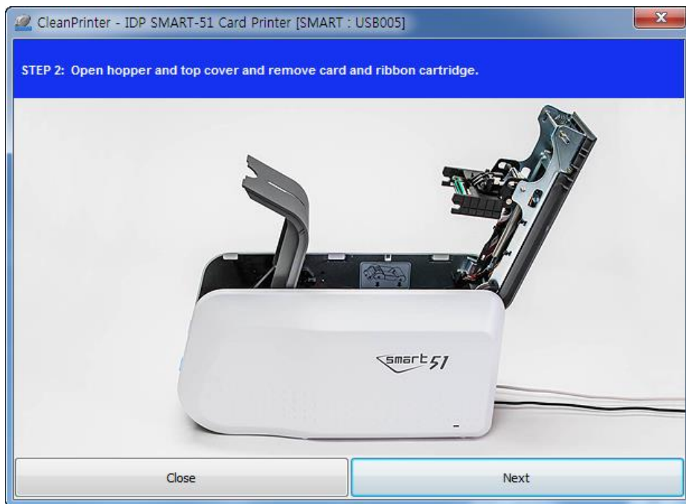
Figure 107 Printer cleaning Step 2
