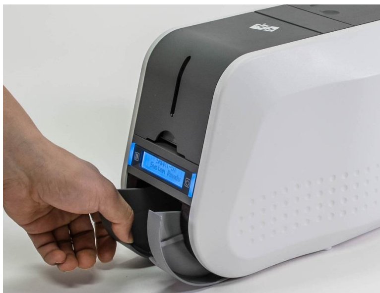
Figure 32 SMART-51 Dividing a stacker
