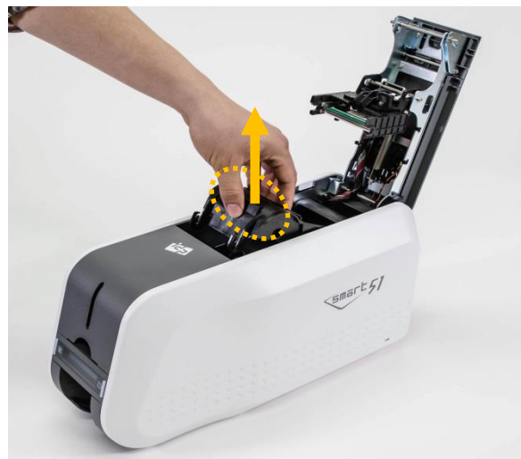
Figure 14 Take out the ribbon cartridge
