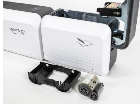
Figure 21 Take out the film cartridge
