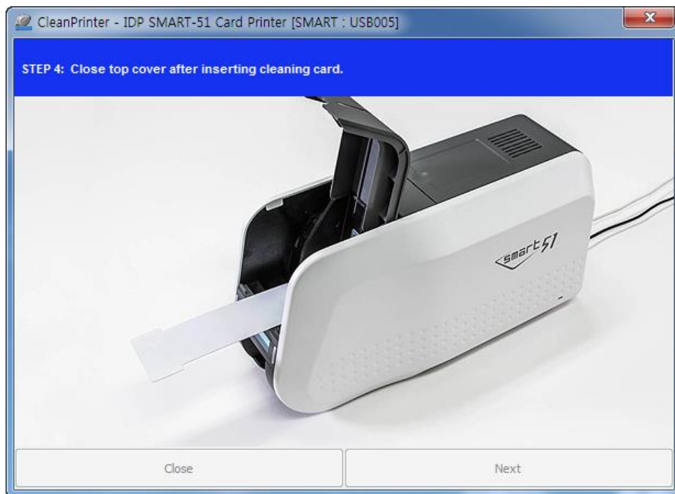
Figure 109 Printer cleaning Step 4
