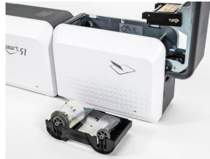
Figure 22 Loading the laminating film
