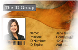
Light or missing transfer on the sides
