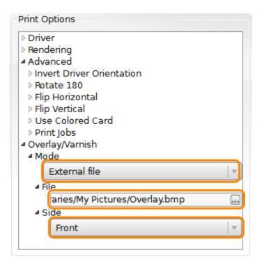
Once **External File** is enabled, **cardPresso** will display an **Overlay/Varnish** tab in the bottom left corner of the **Design View** as shown highlighted in the image below.
