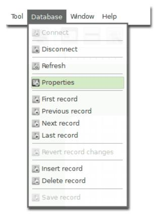
• The Database Properties are mainly used to check the configurations of the connection. Do **not** change them unless necessary.
