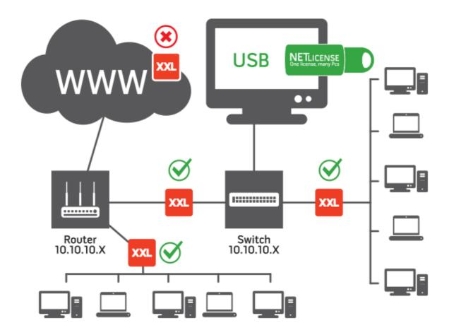
• For best results, the computer with the **Net License Service** should have a Static IP Address. The computer acting as the Net License "Server" does **not** need to have a Server type Operating System.
