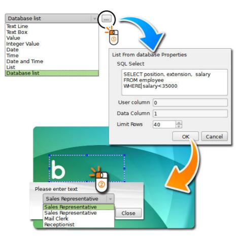
On your combo box is only listed the position field records (User Column 0) that matches the condition (salary<35000). And when the position Mail Clerk is selected the object assume the extension field record of the selected position 6261.
